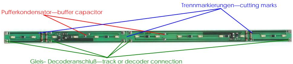
Congratulations for acquiring the analog LED board. The design allows usage in all scales and provide a power supply which can handle even high track volt-ages up to 30V. This board offers multiple cutting marks to adjust the length and stabi-lized brightness independent of the supplied voltage, starting at 6V.
